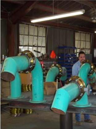
*Miguel Bravo works on turn-out modifications necessary for a float system. All fabrication is done in-house.*
